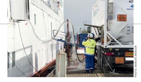
Fuelling Germany's first LNG ship in Bremerhaven. The 94 meter long Borkum ferry "Ostfriesland" owned by AG Ems bunkers 40 cubic meters of LNG
