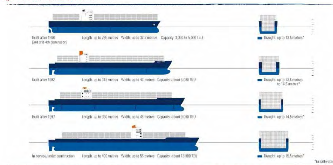
Figure 21: Growth in dimensions of container vessels
